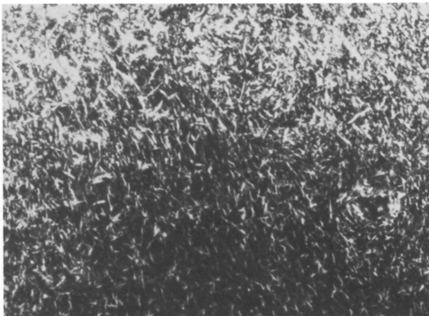
Figure 5: Optical polarization micrograph for a polyketone based on fluorene and 1,10-decanedicarboxylic acid (No. 7, Table I); smectic bâtonnets at 135°C (heating cycle, 80x).
